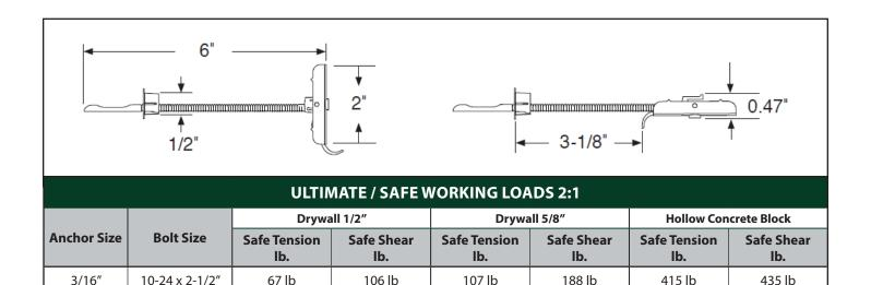
2:1 Loads may vary according to the quality of the drywall or concrete hollow block.
