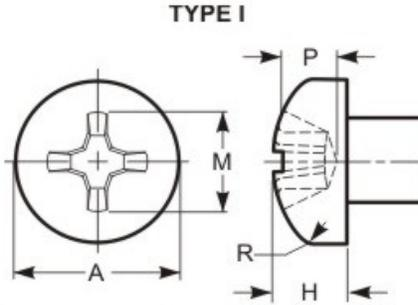
This type of recess has a large center opening, tapered wings, and blunt bottom, with all edges relieved or rounded.
