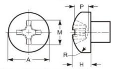
This type of recess has a large center opening, tapered wings, and blunt bottom, with all edges relieved or rounded.
