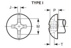
This type of recess has a large center opening, tapered wings, and blunt bottom, with all edges relieved or rounded. A slot crosses the head aligned with one pair of wings.
