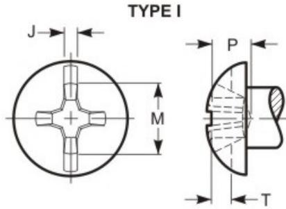
This type of recess has a large center opening, tapered wings, and blunt bottom, with all edges relieved or rounded. A slot crosses the head aligned with one pair of wings.
