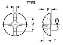
This type of recess has a large center opening, tapered wings, and blunt bottom, with all edges relieved or rounded. A slot crosses the head aligned with one pair of wings.
