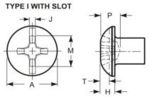
This type of recess has a large center opening, tapered wings, and blunt bottom with top edges relieved or rounded. A slot runs parallel to one pair of recess wings.
